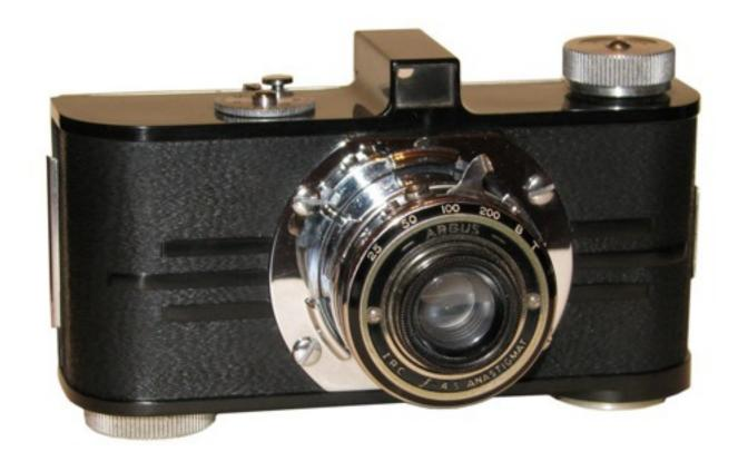
**Description** 35mm cartridge camera with bakelite body. Argus Anastigmat f4.5/50mm in collapsible mount. Early models have fixed pressure plate, sprockets on one side of film. Later models have floating pressure plate and sprockets on both sides. Of early types, the first 30-35 thousand were made before a tripod socket was added to the bottom and the rewind knob thickened to match. Originally advertised in the following color combinations: black/chrome, gray/gunmetal, ivory/gold.
