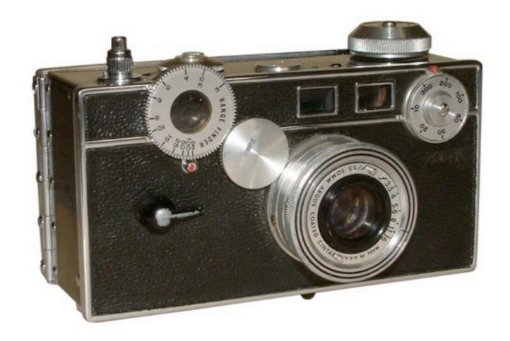
**Description** Like the "C", but the rangefinder is coupled. Introduced just after the model C in 1938. An Early "brick", also found with all metal trim in high polished-chrome finish.
