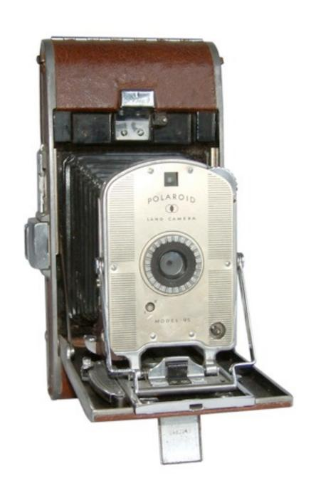
**Description** The first instant picture camera. Folding design. Aperatures f11-f45, speeds 1/8-1/60s, linked and controlled by single dial, numbered 1-8. Took Polaroid's first instant rollfilm to make sepia pictures in around a minute. Early models had rigid viewfinder mast, later models had a folding mast.
