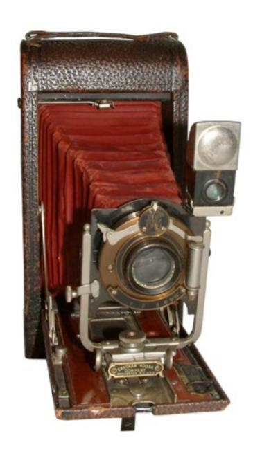
**Description** Vertical folding-bed camera for 3 1/4 X 5 1/2 exposures on 122 rollfilm (introduced for this camera). Flat, rectangular front door. Red bellows (black after August 1912). Polished-wood insets on bed.
