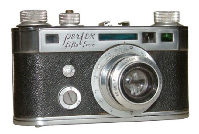
**Description** Wollensak Velostigmat lens. Focal-plane shutter, 1-1250, B, sync. CRF. Extinction meter and exposure calculator.
