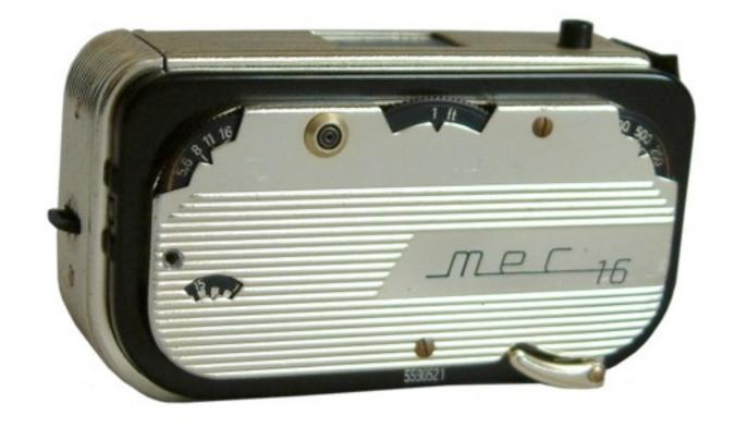
**Description** By Feinwerktechnik, Lahr, Germany for 10x14mm exposures on 16mm film in cassettes. Pull-out finder protects double exposure. Lenses: Color Ennit 2,8/20 & Heligon 2/22 all metal focal plane shutter 1/30 - 1/1000 Sek.
